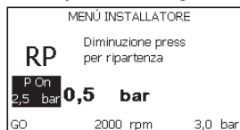
Figure 17: Setting the restart pressure
