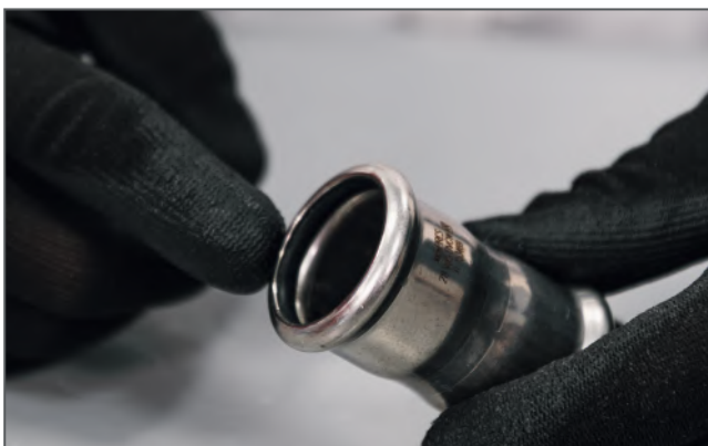
Controllo O-ring / Checking the sealing ring
